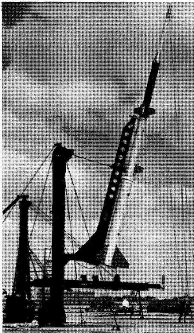
FIGURE 380. Model of Polaris nose cone, shown on four-stage Honest John booster for heat-transfer test to Mach 10, October 6, 1958.
