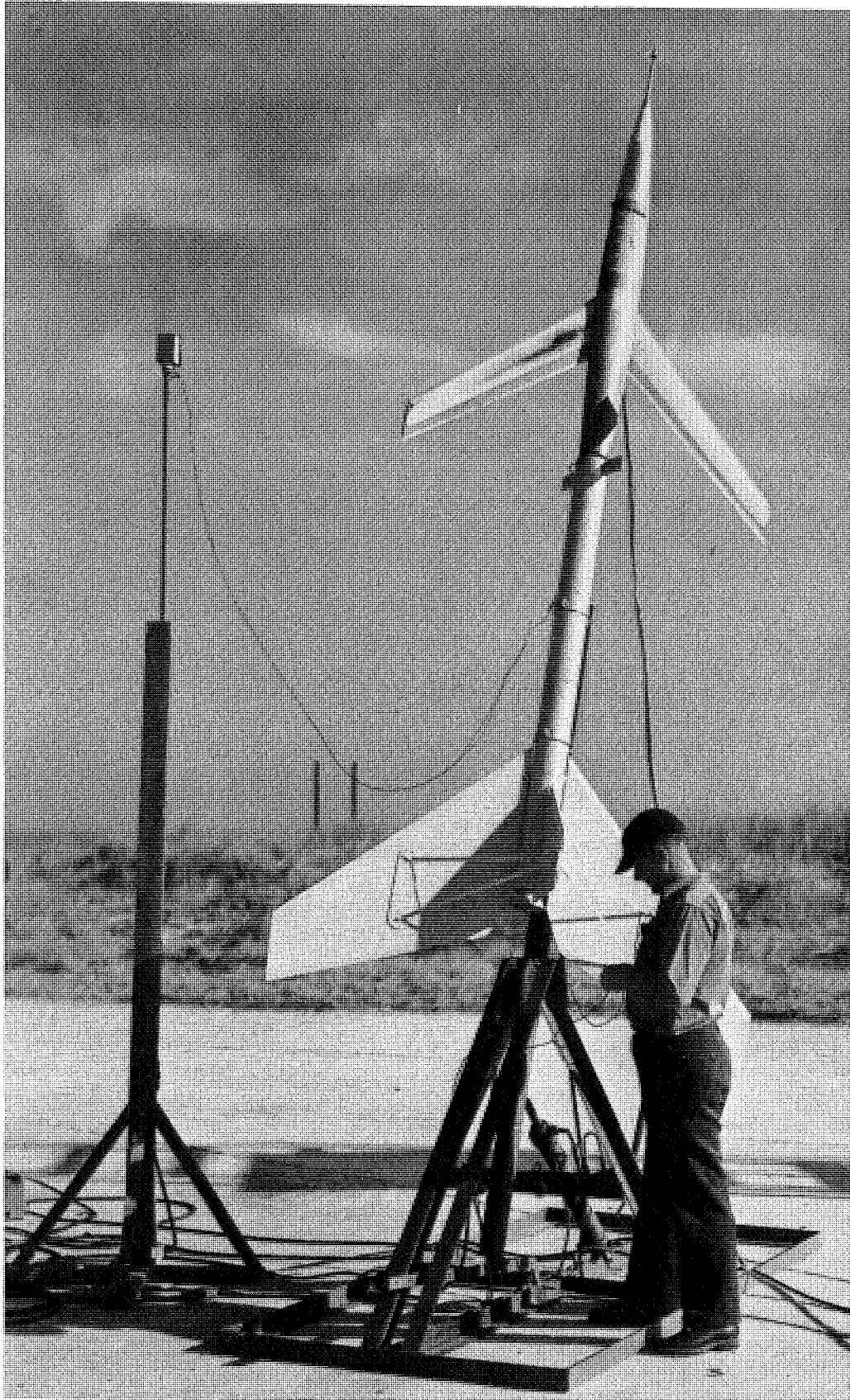
FIGURE 237. Technician Ed Matthews connects firing leads to 65-HVAR booster for E31 aero-elasticity model, November 14, 1952.
