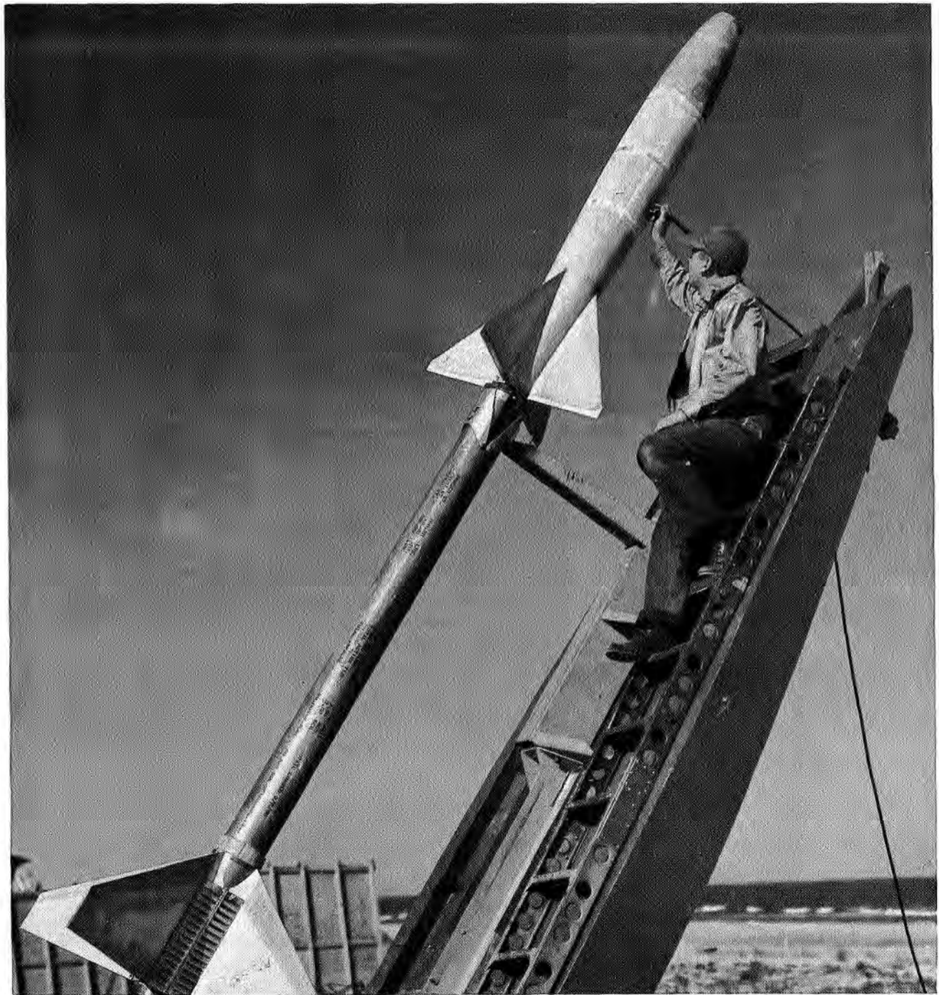
FIGURE 111. First F26 transonic inlet model with Deacon booster. Project engineer R. I. Sears checks external-power plug, May 23, 1950.
