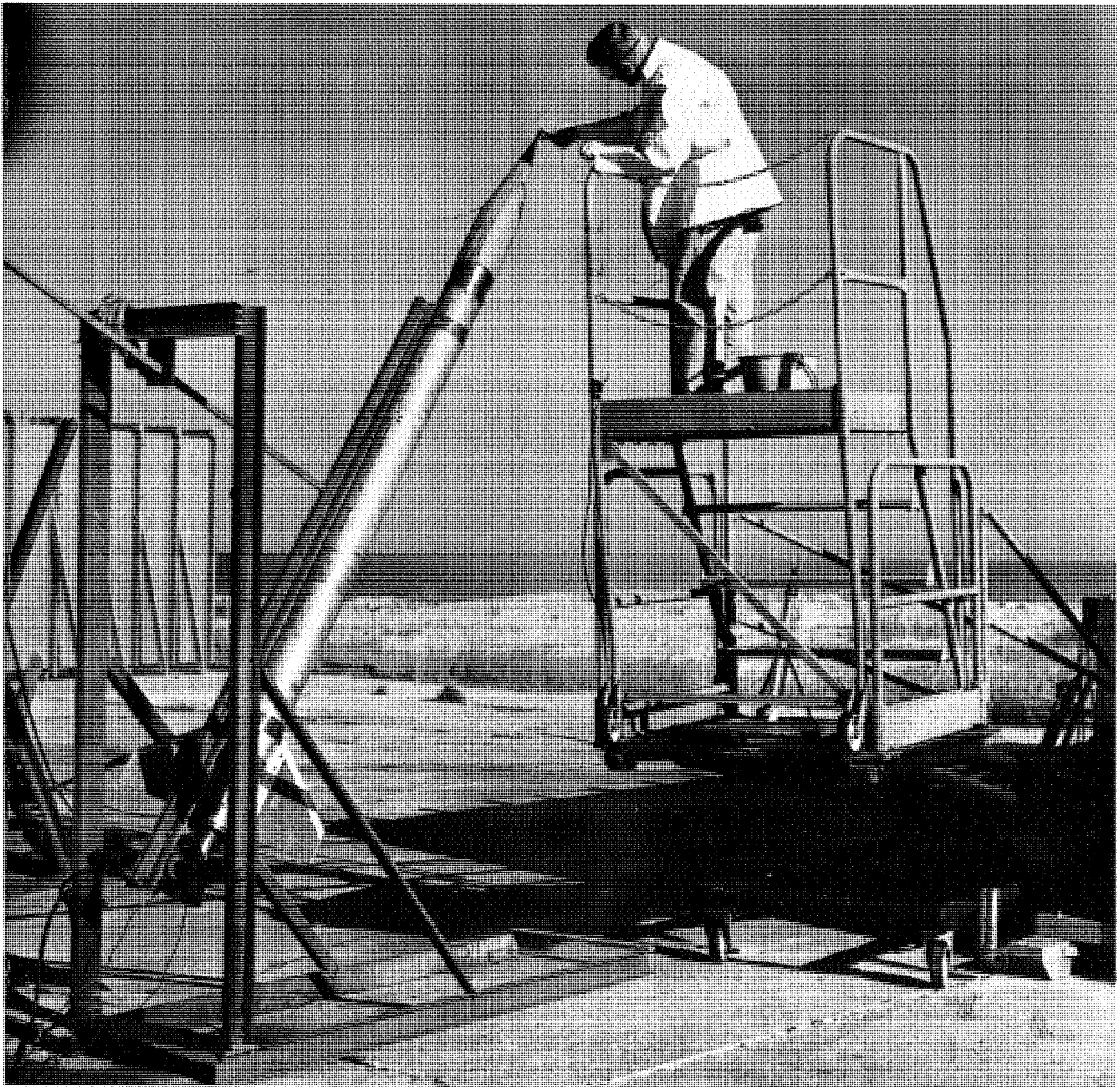
FIGURE 253. Technician pours PS smoke chemical into nose cone of Deacon-powered smoke rocket used by Naval Ordnance Laboratory for initial test at Wallops, October 11, 1955.
