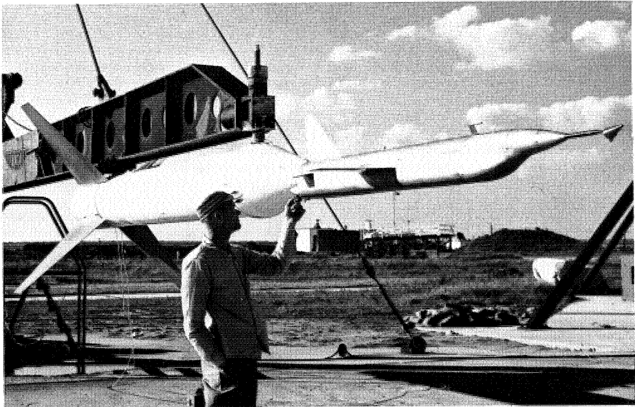
FIGURE 271. Technician Durwood Dereng installs firing leads to one of two Loki motors in enlarged fuselage of an E15 longitudinal stability model, shown with a Nike booster, September 8, 1958.
