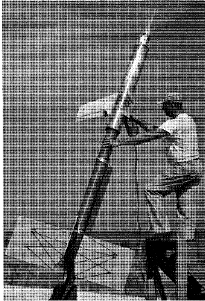
FIGURE 267. Technician W. A. Roberson prepares to pull the external-power plug from a rocket model designed to investigate aileron buzz. The model is shown in launch position at Wallops, July 9, 1951.
