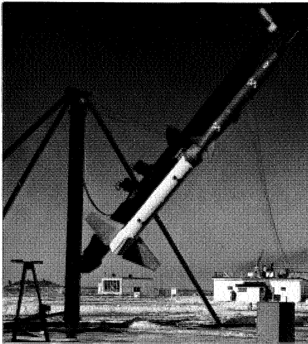
FIGURE 381. Temco Corvus guided missile ready for flight test at Wallops with Honest John booster, December 18, 1958.
