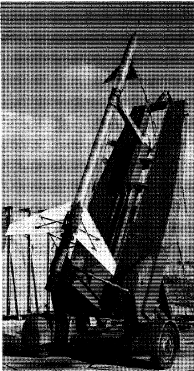
FIGURE 233. Rocket model of AGARD Model 2 with Deacon booster at Wallops, November 27, 1956.
