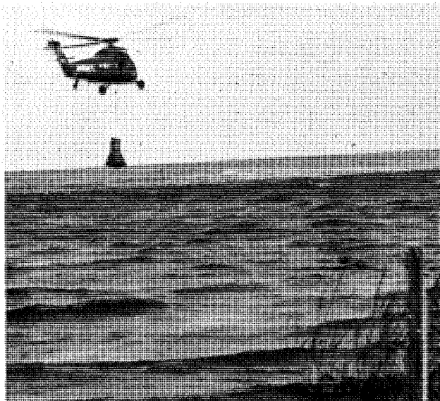
FIGURE 425. Marine helicopter retrieves boilerplate Mercury test capsule from water after air-drop from C-130 airplane, November 25, 1958.
