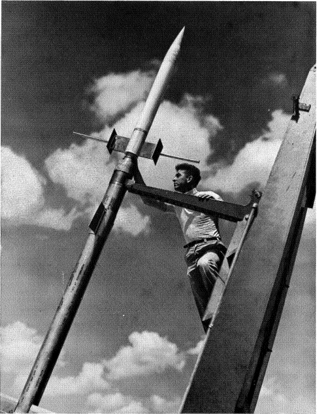
FIGURE 131. Technician William Ferguson adjusts Deacon booster adapter on E2 model at Wallops, May 7, 1951. Model was used in basic research on drag of cylinders.
