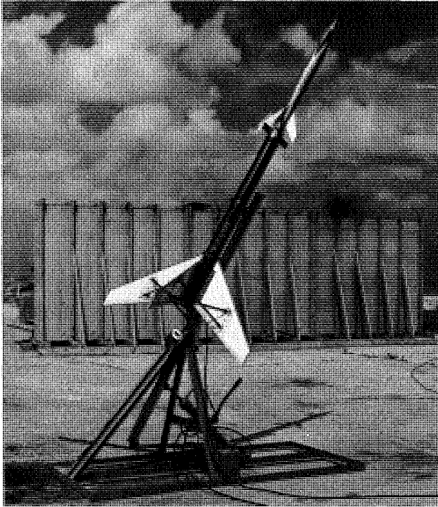
FIGURE 304. Rocket model with canopy and fuselage area-rule indentation on parabolic body. Model is shown in mounted position at Wallops, June 29, 1955.
