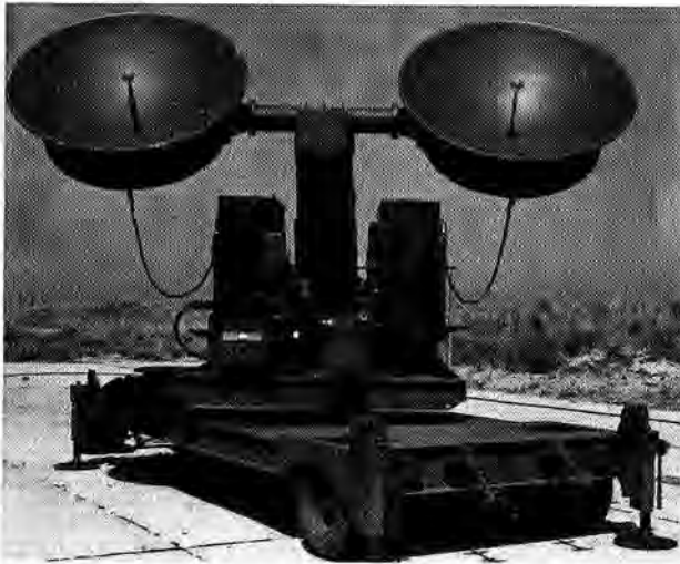
FIGURE 176. Sperry model 10C Doppler Velocimeter at Wallops, June 1, 1954.
