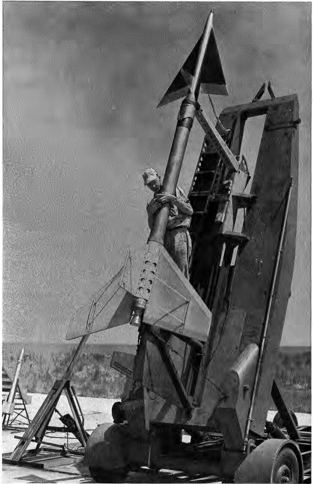
FIGURE 102. Model of Northrop Boojum MX-775B supersonic strategic missile shown with Deacon booster on launcher at Wallops, August 2, 1951. Technician Durwood A. Dereng measures elevation angle.
