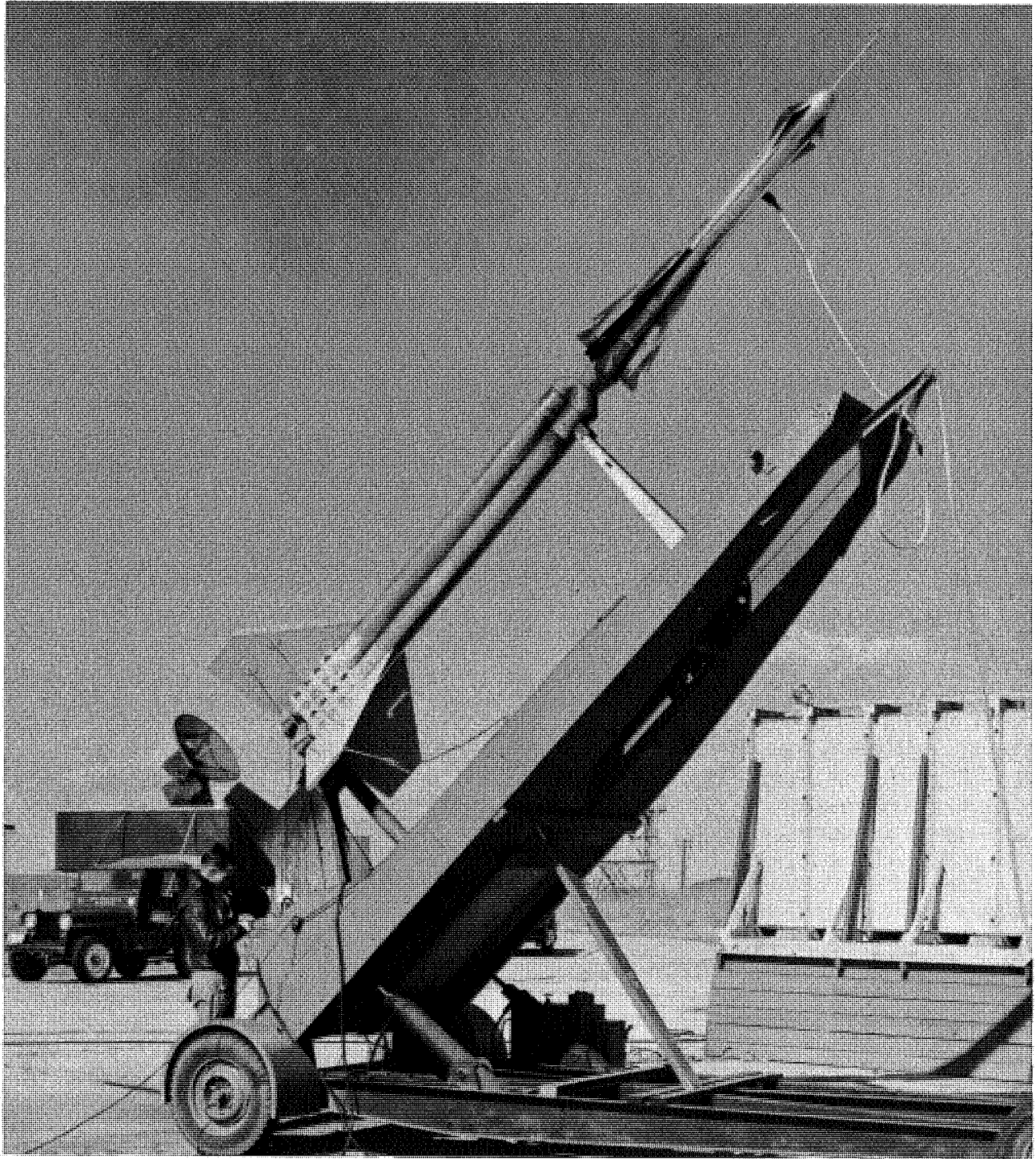
FIGURE 231. Technician Roy Hindle connects firing leads to double Deacon booster for Hughes Falcon guided missile, March 5, 1953.
