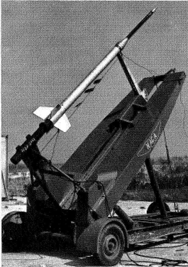
FIGURE 296. Cajun-Loki test vehicle for research in aerodynamic ignition of metallic cone. Vehicle is shown on mobile launcher, August 1, 1956.
