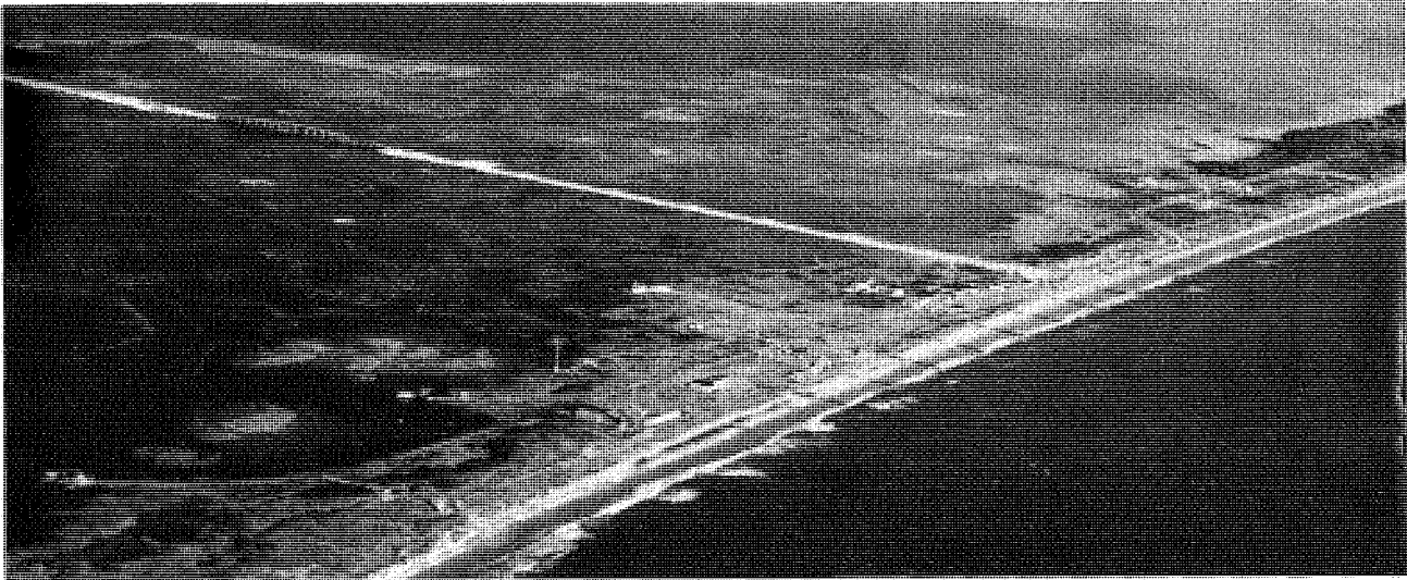
FIGURE 412. Aerial view of Wallops Island, December 1959, showing groins extending into the ocean from the seawall between the Assembly Shop area and the causeway.
