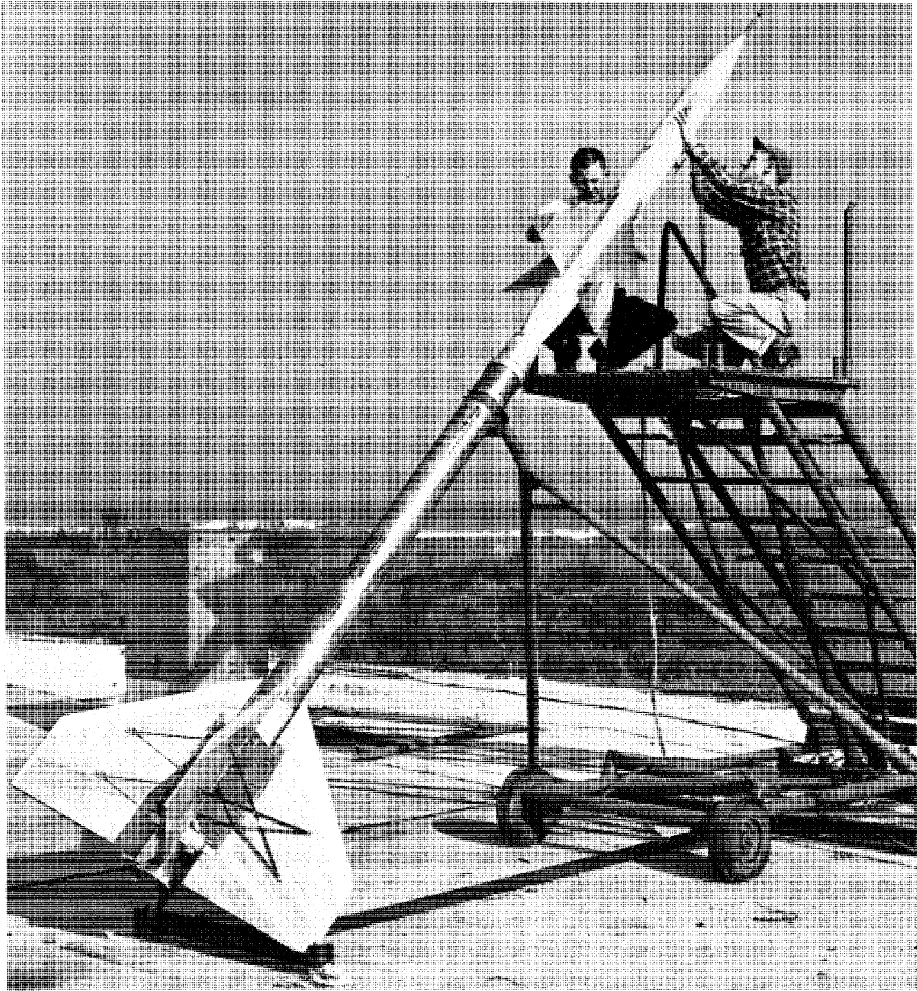
FIGURE 168. Technicians Nat Johnson and Durwood Dereng make final check of D8 aerodynamic control hinge-moment model on crutch launcher at Wallops, October 2, 1950.
