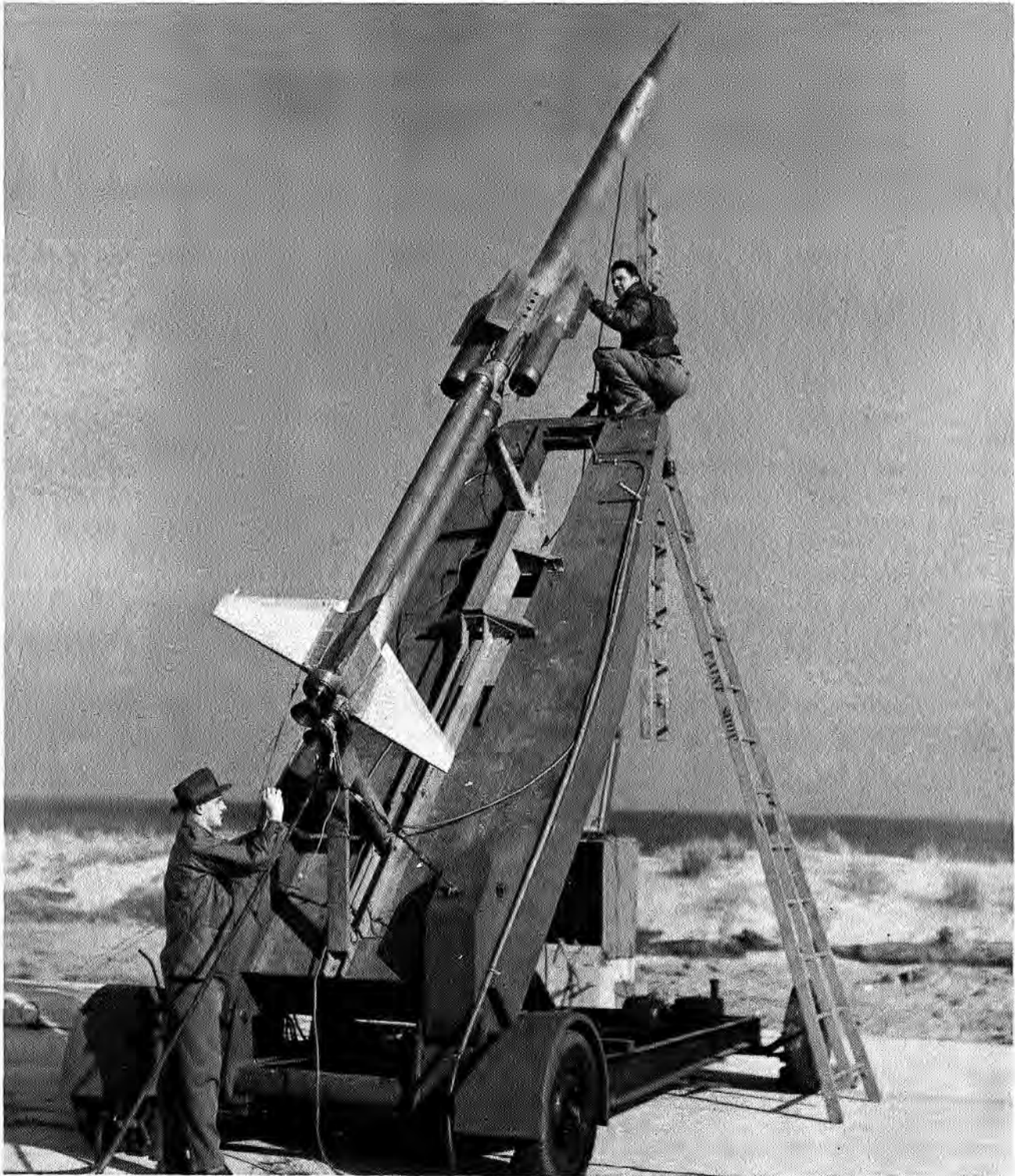
FIGURE 108. First successful F23 twin-engine ramjet vehicle with double Deacon booster. Project engineer H. R. Dettwyler, on ladder, inspects one of the engines while engineer J. E. Stevens examines electrical wiring, March 24, 1950.
