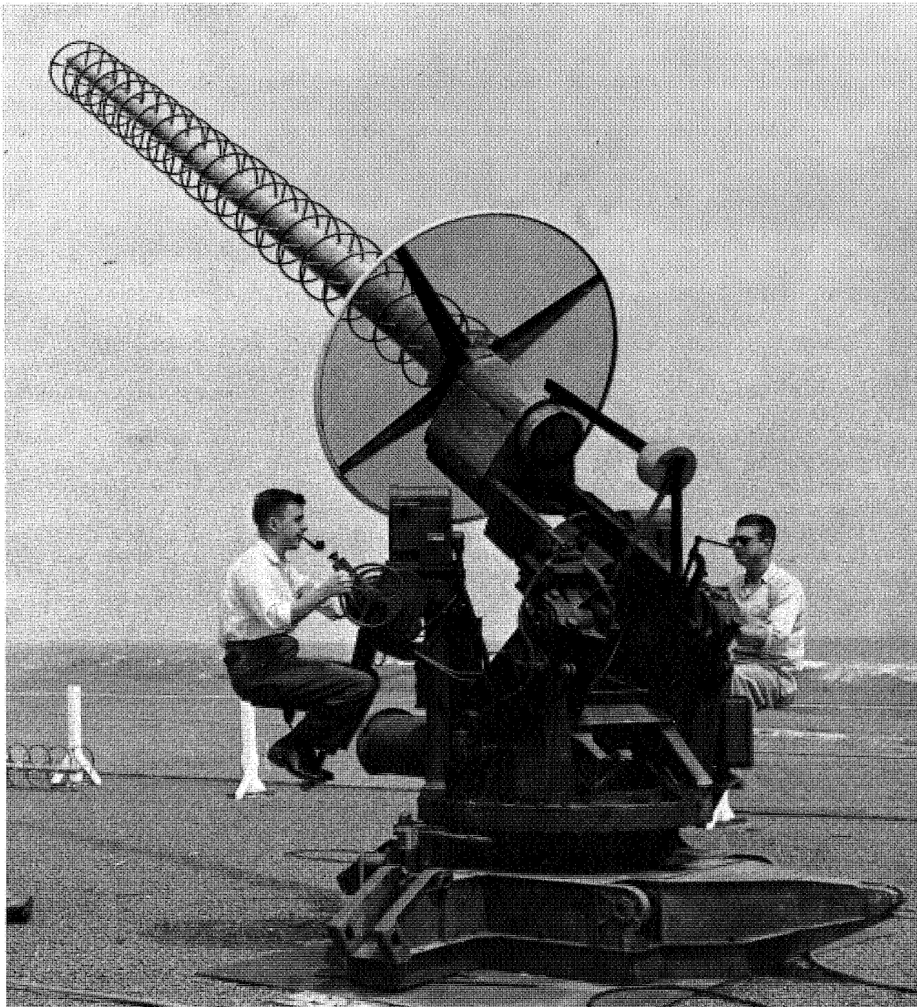
FIGURE 350. Twenty-turn helical antenna mounted on roof of Control Center 1. View shows J. B. Aaron (left) and R. R. Johnson pointing antenna at model in flight.
