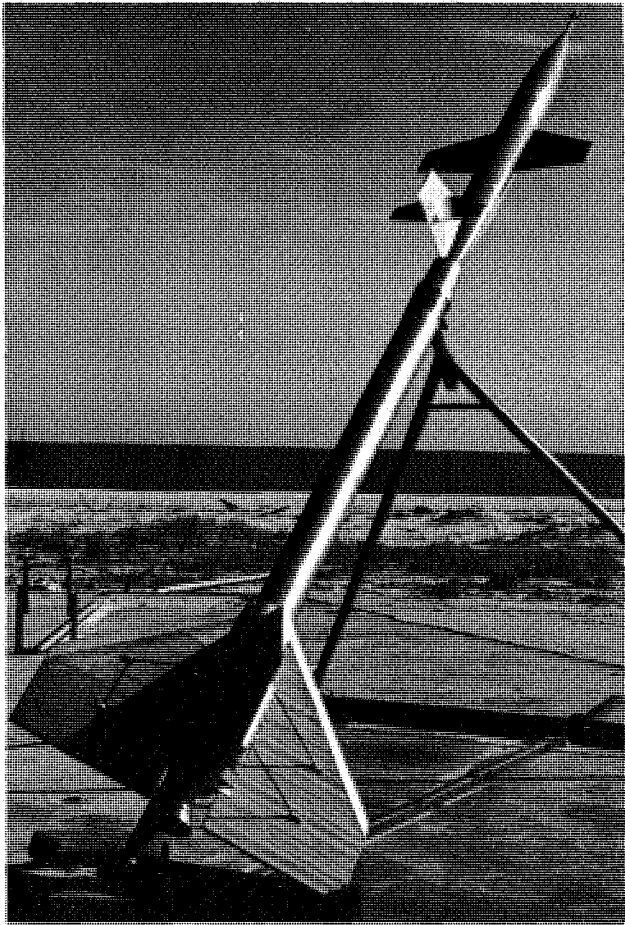
FIGURE 82. Typical E15 research rocket model used to investigate dynamic longitudinal stability. Model is shown ready for launching on February 2, 1949.
