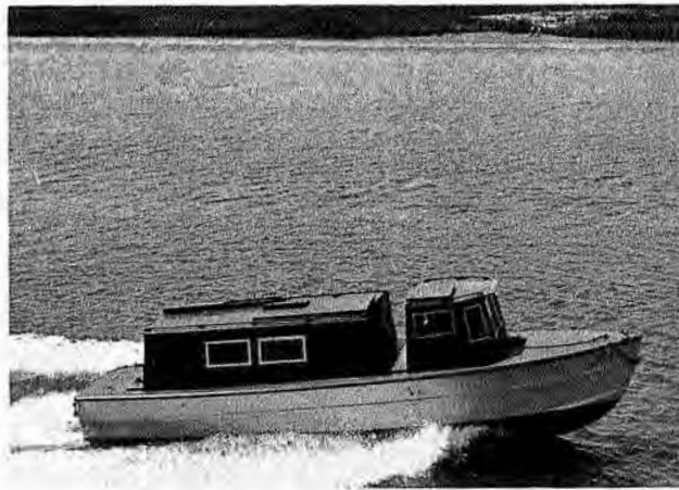
FIGURE 12. Navy 26-foot plane personnel boat shown operating in the Wallops-Island-to-mainland waterway. Craft was fitted with cabins for passengers and crew.
