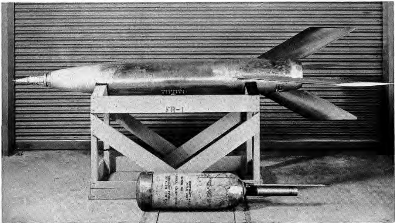
FIGURE 51. First low-acceleration rocket-propelled flutter model, FR-1, March 5, 1947.
