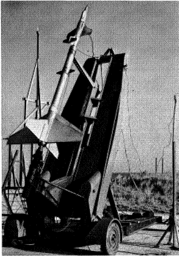
FIGURE 222. Model of Lockheed XF-104 Starfighter, shown with Deacon booster at Wallops, January 4, 1954.
