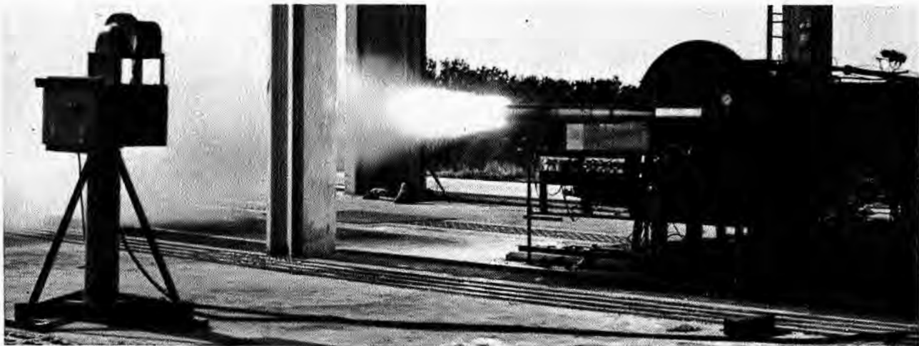
FIGURE 110. Typical F23 ramjet engine during operational test in Wallops Preflight Jet.
