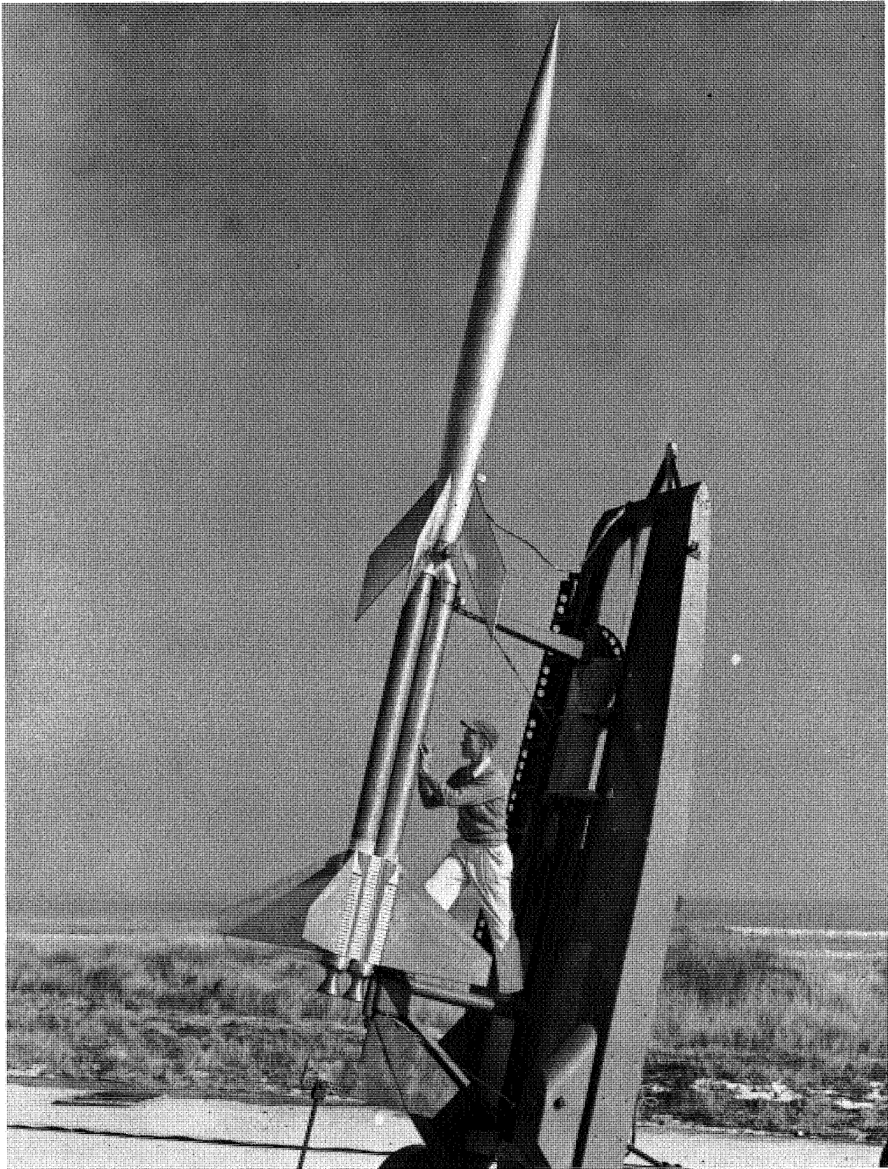
FIGURE 134. Technician Durwood Dereng measures elevation of double Deacon booster prior to launch of RM-10 research model at Wallops, February 6, 1951.
