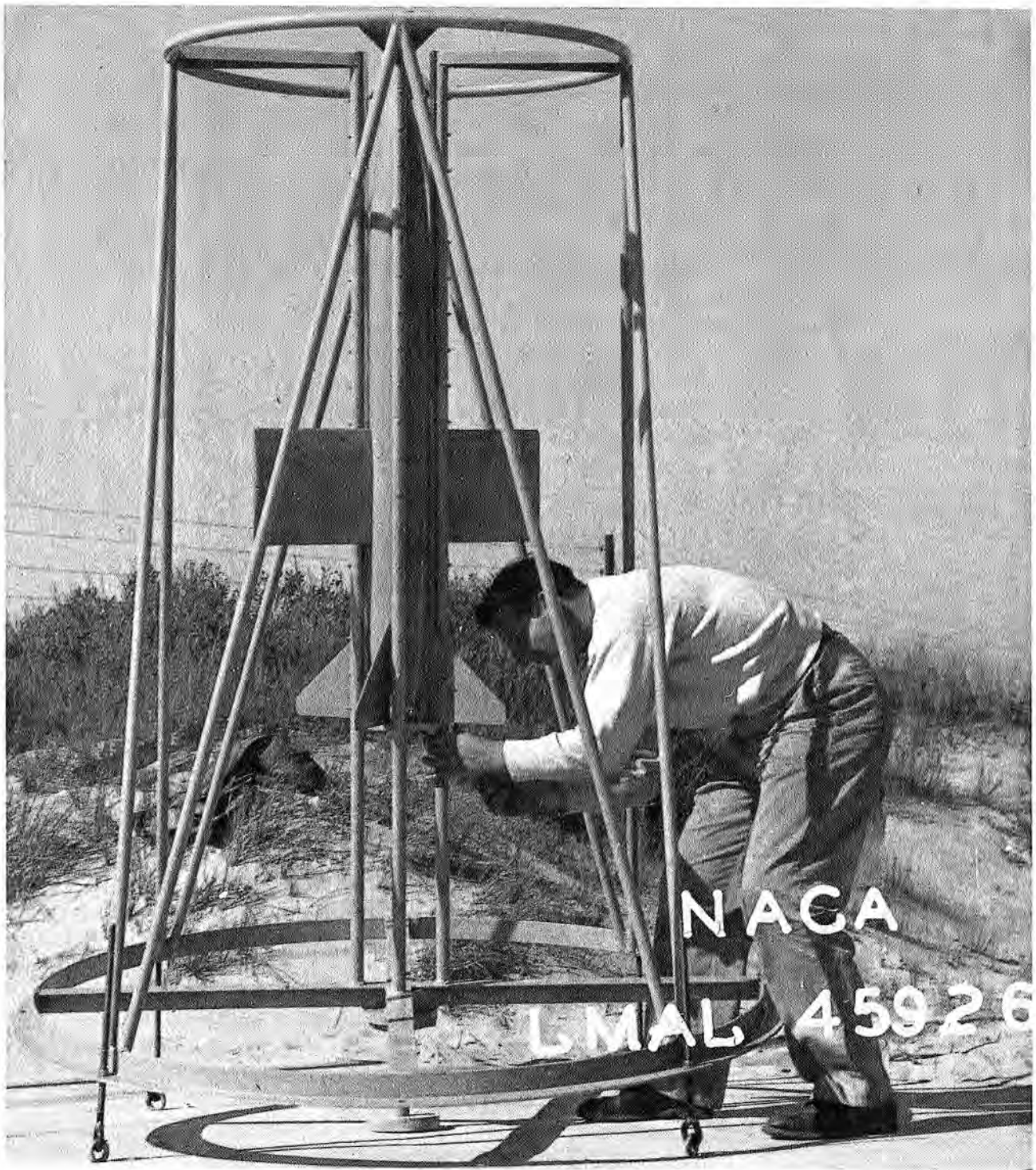
FIGURE 33. Project engineer Sidney Alexander adjusts typical RM-2 model on its special launcher at Wallops Island, October 1945.
