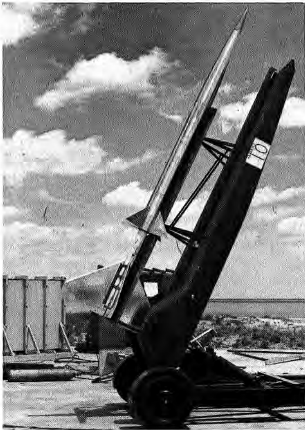
FIGURE 99. Sparrow guided missile model and HVAR booster mounted on launcher.
