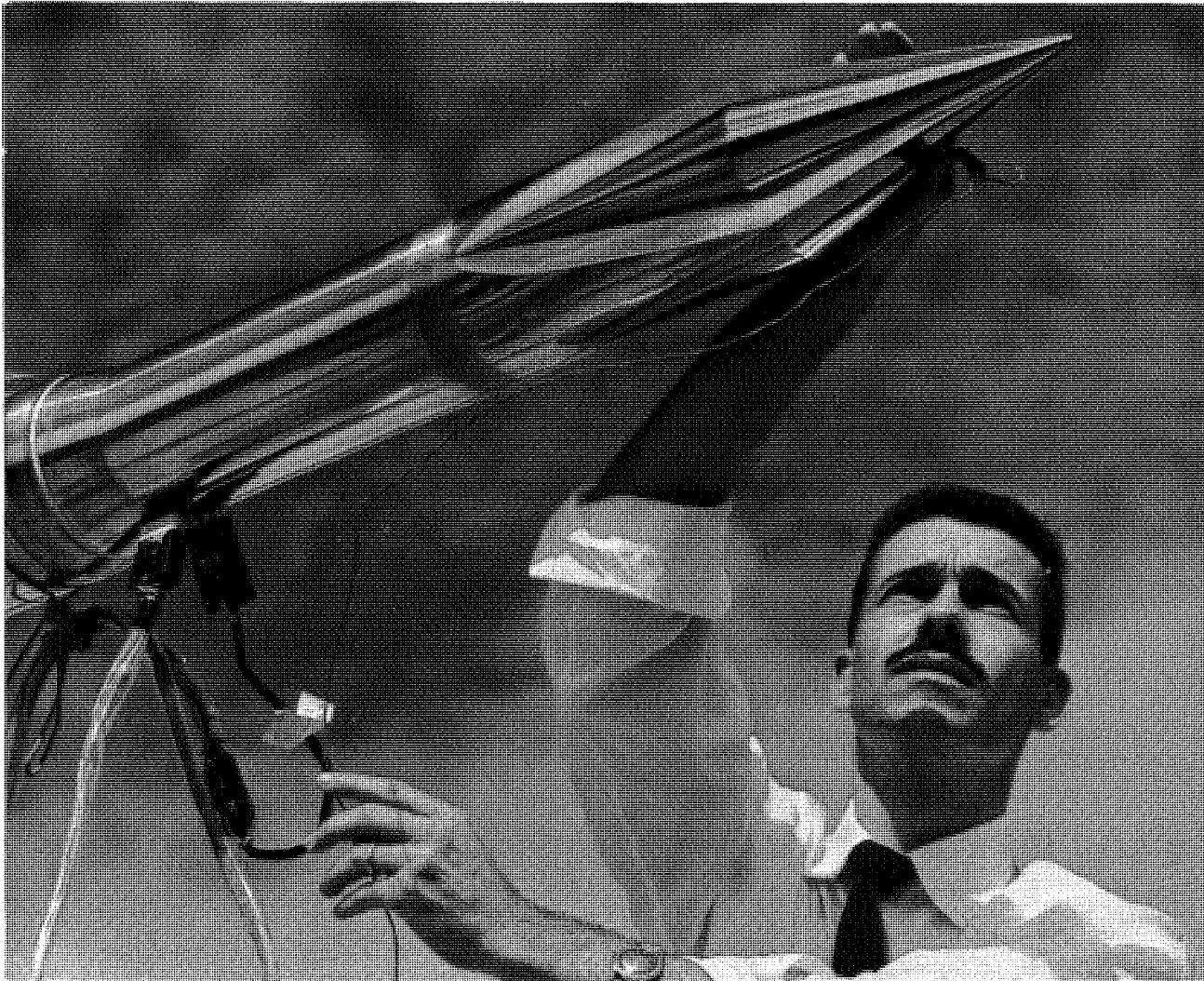
FIGURE 372. Engineer Glenn Burton examines simulated delta-wing glide-rocket model with conical body at an angle of attack (photograph of October 8, 1957).
