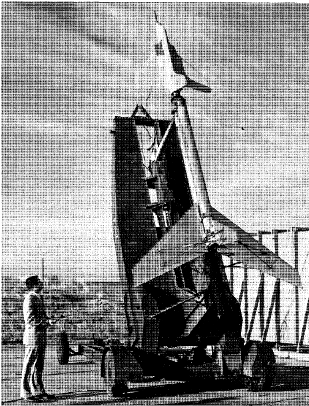
FIGURE 297. Rocket model of Douglas F5D-1 airplane, shown on mobile launcher with double Deacon booster, December 13, 1956.
