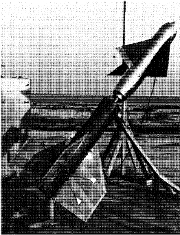
FIGURE 80. Monsanto ACL-1 rocket motor booster with 1/8-scale model of Convair XF-92 airplane ready for launching at Wallops Island, November 7, 1947.
