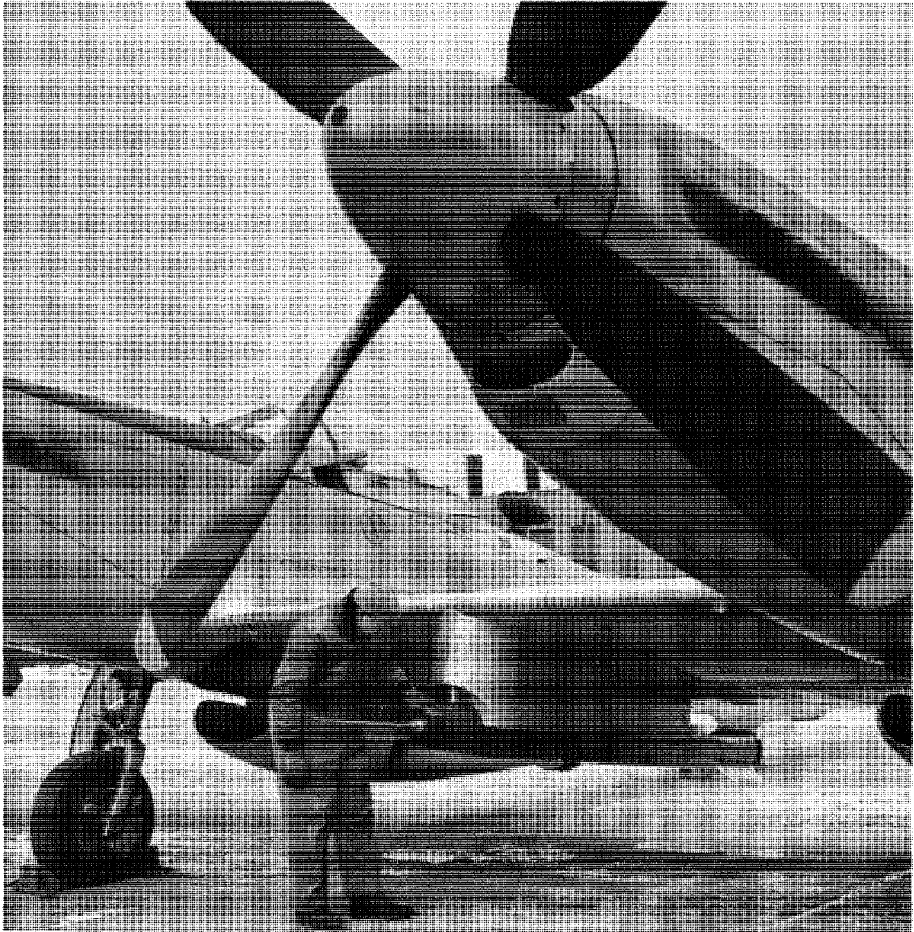
FIGURE 200. Lewis engineer Scott H. Simpkinson examines 9.75-inch high-energy ramjet engine on North American F-82 airplane prior to flight to Wallops for air launch on February 12, 1954.
