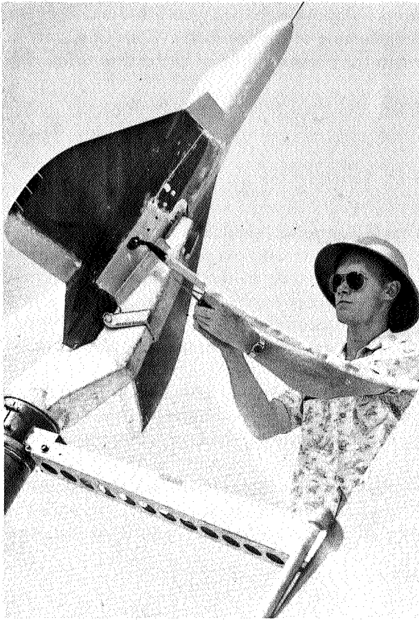
FIGURE 154. Technician Durwood Dereng makes final adjustment of booster adapter on model of Douglas XF4D-1 Skyray airplane on mobile launcher at Wallops, June 27, 1951.
