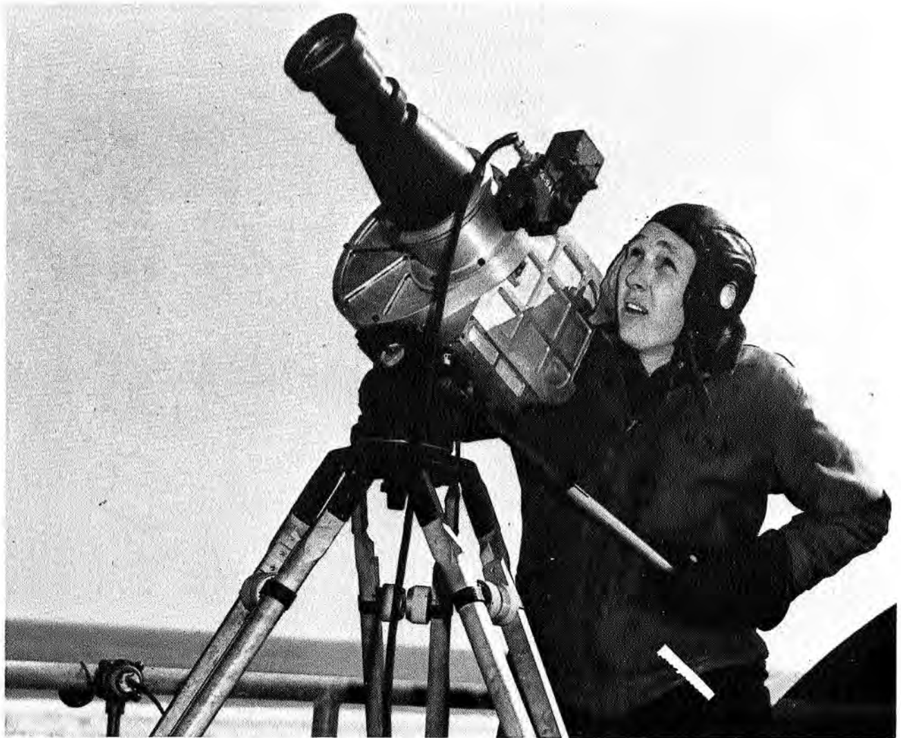
FIGURE 95. Photographer Donald S. Foster operates first Hulcher sequence camera at Wallops. Camera is shown mounted on tracking tripod.
