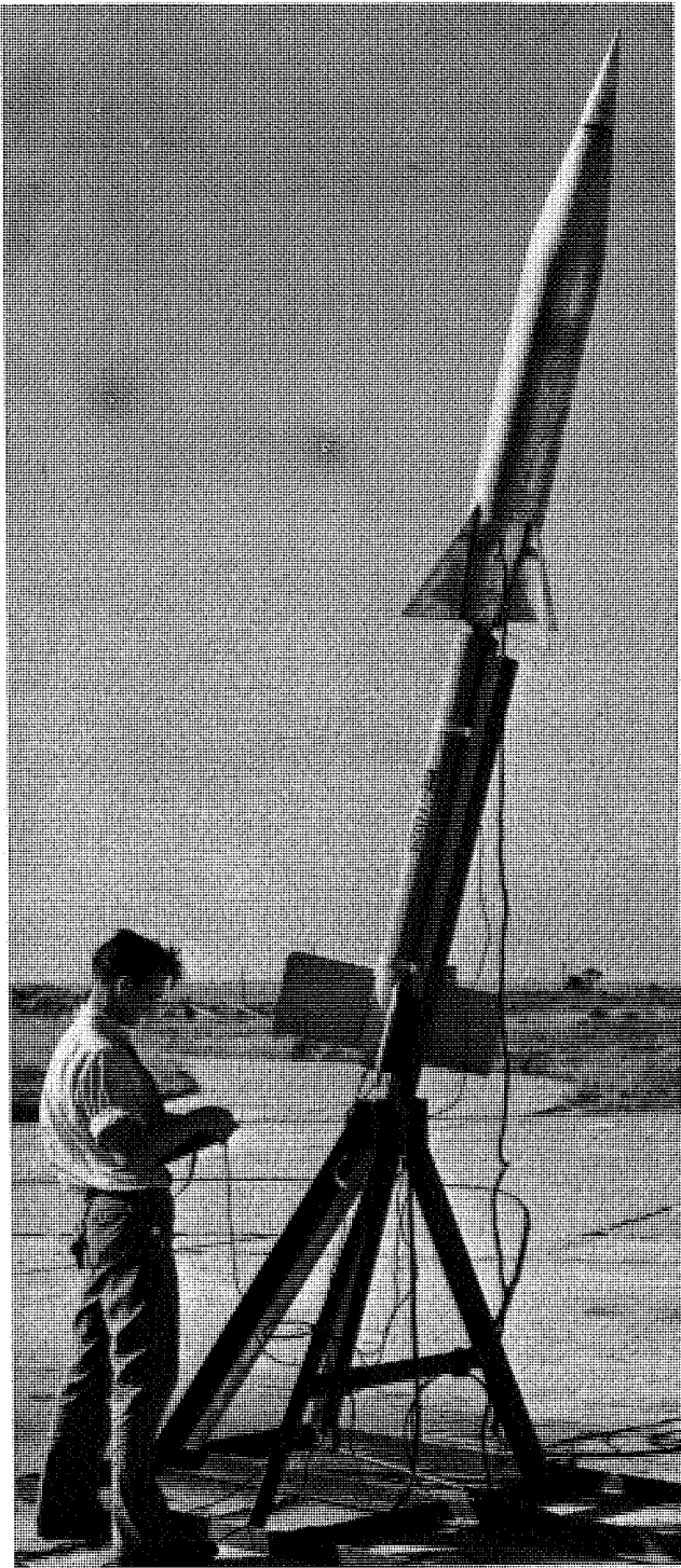
FIGURE 235. Technician Roy Hindle connects firing leads to HVAR booster for F12 jet-effects flight model, June 3, 1952.
