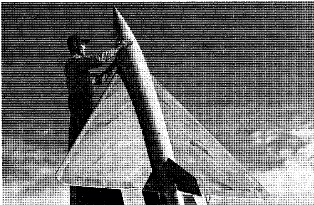
FIGURE 137. Technician Durwood Dereng prepares to pull the external-power plug from an E17 drag-research model at Wallops, September 8, 1950.
