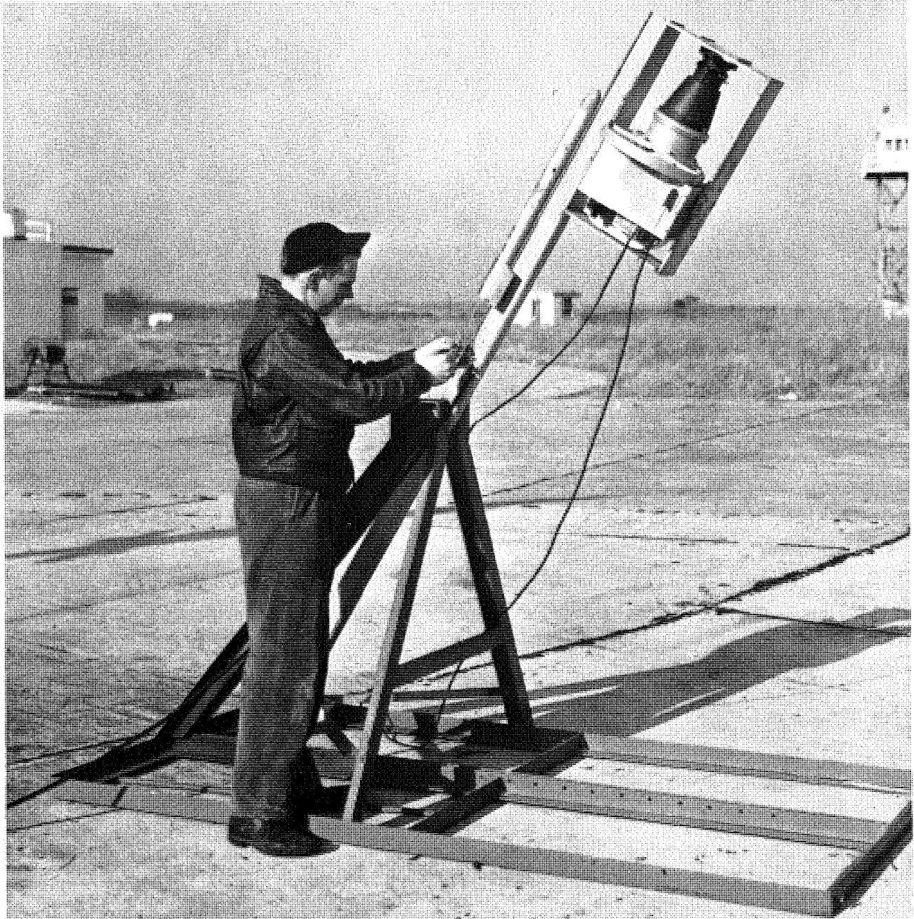
FIGURE 167. Photographer W. Carr connects firing leads on a 2.25-inch rocket with twisted monoplane fins. Hulcher camera is shown in position to record dispersion of rocket in flight, December 22, 1952.
