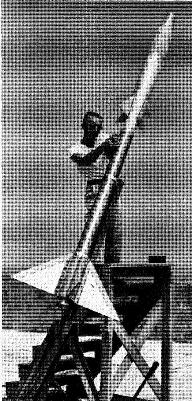
FIGURE 202. Technician Franklin Forbes measures elevation angle of HPAG booster for F26 inlet model on rail launcher, July 18, 1951.
