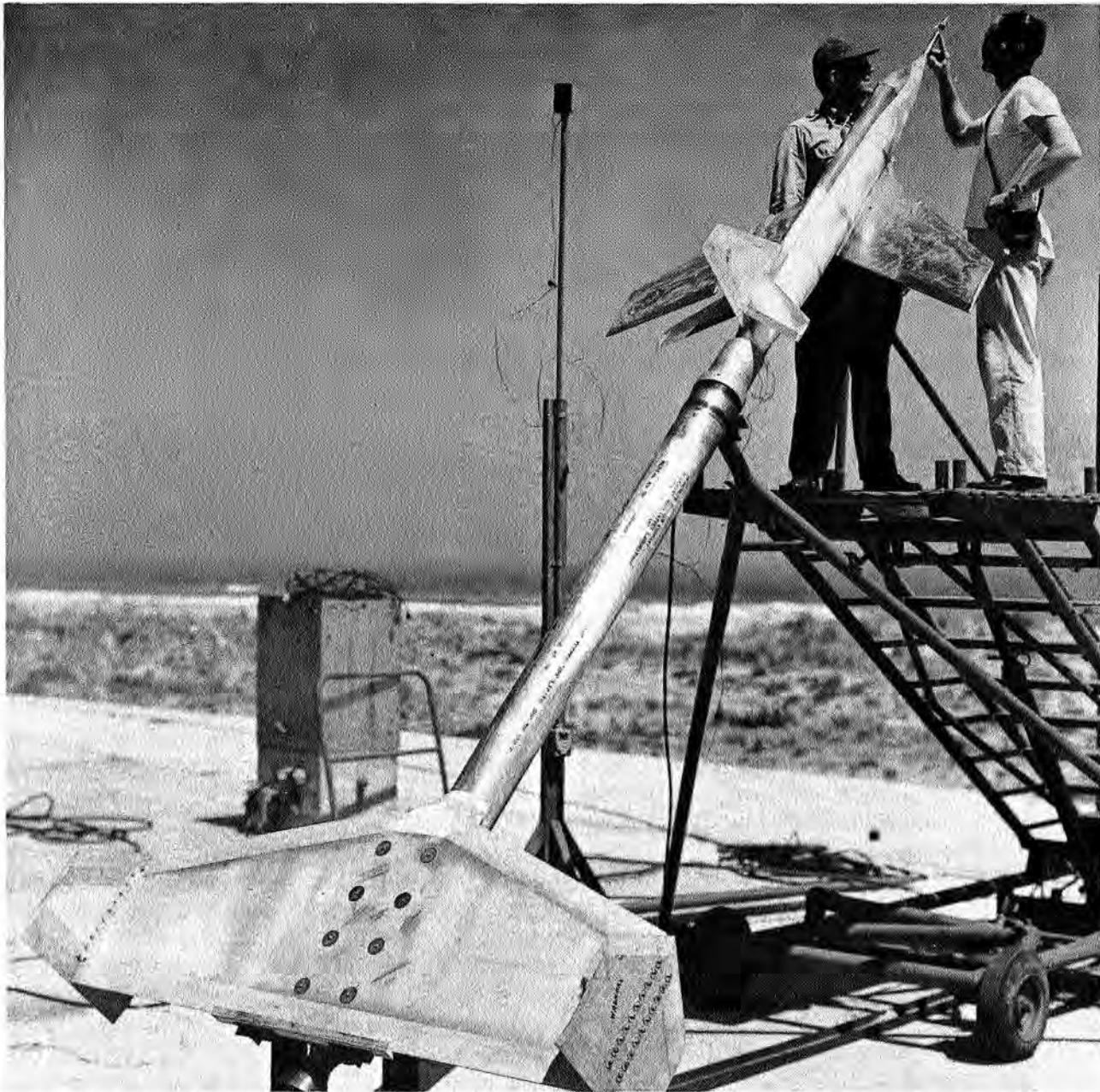
FIGURE 105. Model of Bell X-2 research airplane with Deacon booster on crutch launcher. Project engineer C. T. D'Aiutolo, at left, and technician Thomas Bigger inspect angle-of-attack instrument, May 12, 1950.
