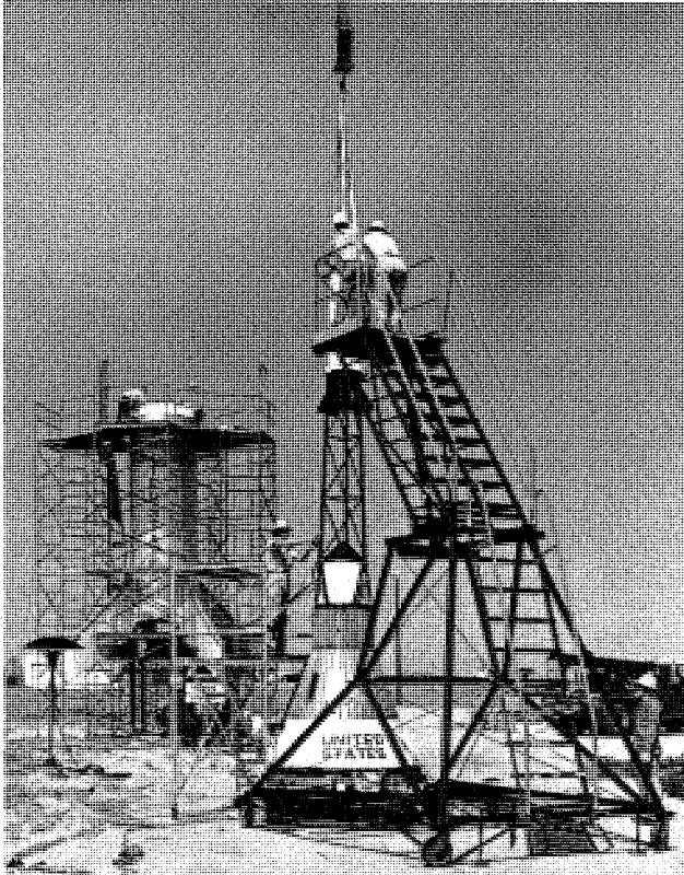
FIGURE 432. Technicians attach escape tower to prototype Mercury capsule prior to assembly with Little Joe launcher, August 20, 1959.
