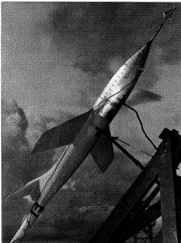
FIGURE 155. Model of Douglas D-558-II research airplane flown on August 6, 1952, to investigate coupled pitch and yaw motions. View shows vane mounted on nose boom to measure angle of attack and angle of sideslip.
