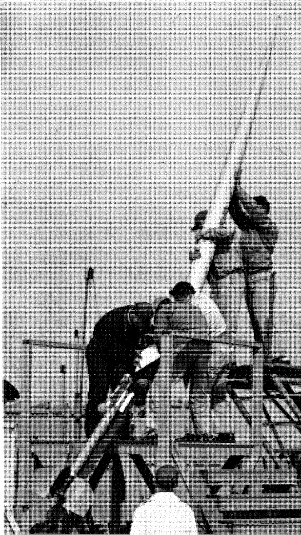
FIGURE 129. Work crew prepares to connect E2 parabolic body of fineness ratio 24.5 to its booster on the rail launcher at Wallops, May 18, 1950.
