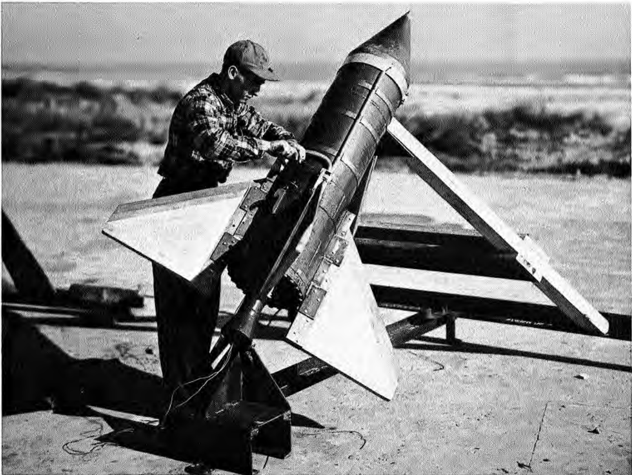
FIGURE 49. Technician Phil Mears adjusts Aerojet T27 jato rocket motor for flight test at Wallops, November 18, 1948.
