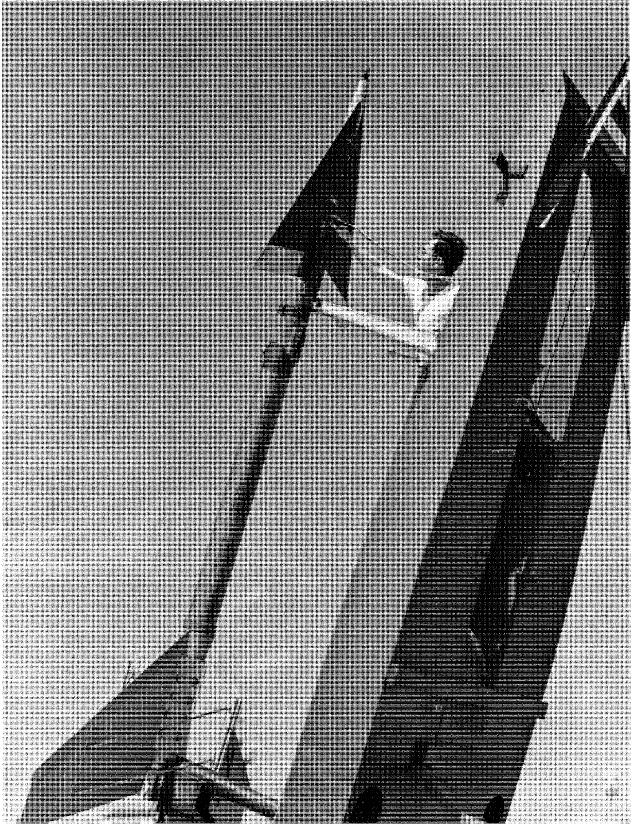
FIGURE 120. Engineer R. A. Arbic examines external-power plug leading to model of Northrop Boojum missile on launcher at Wallops.
