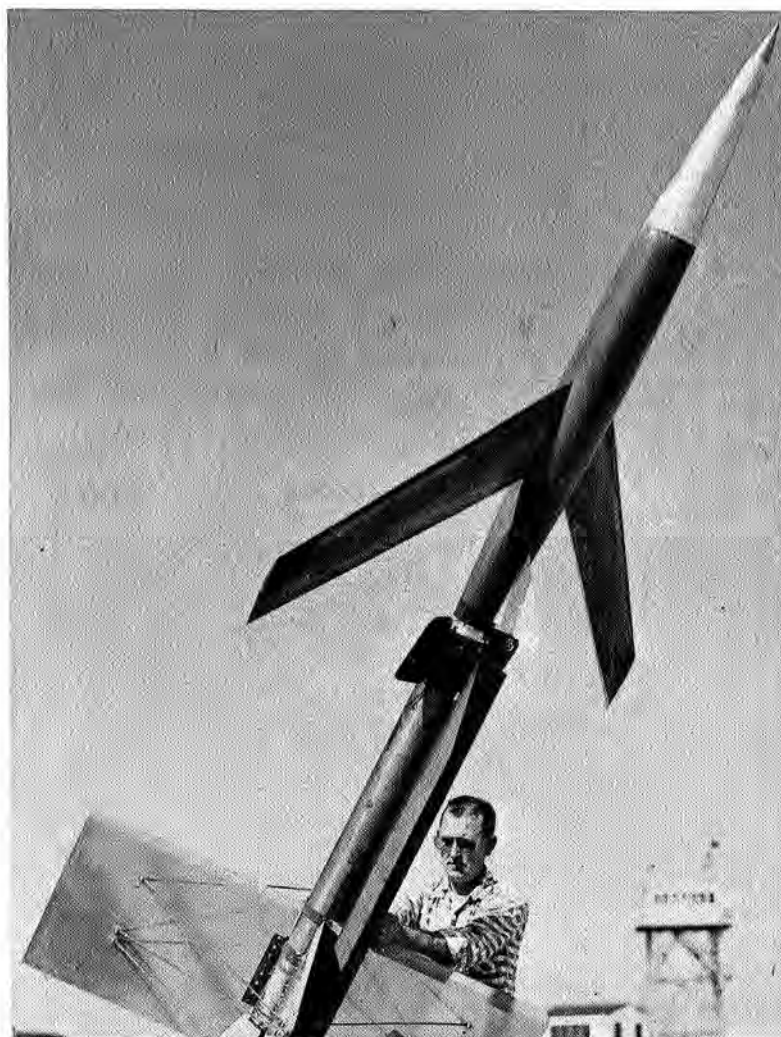
FIGURE 113. View of F25 transonic drag model with basic wing H, mounted on rail launcher with HVAR booster, October 10, 1950. Propulsion technician Nat Johnson connects firing leads.
