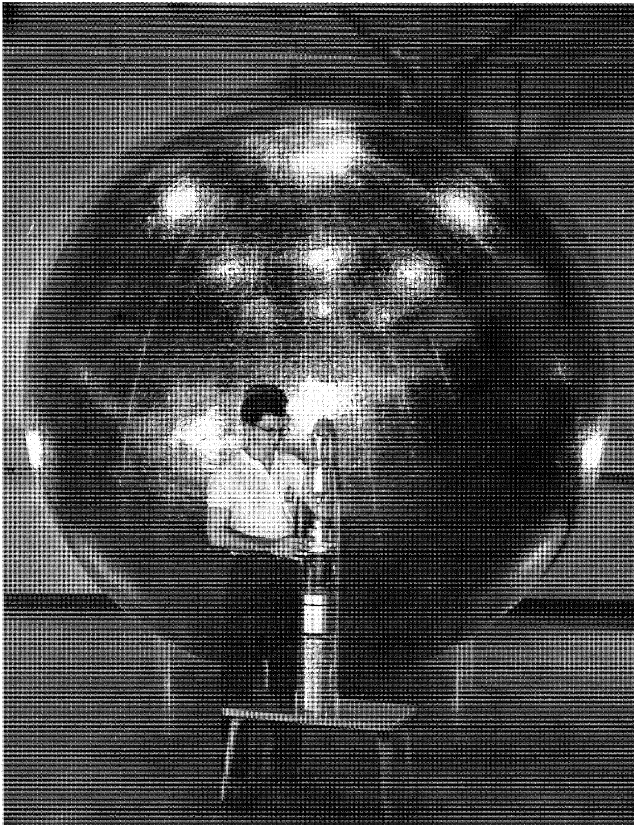
FIGURE 402. Engineer W. D. Nowlin with one of the 12-foot inflatable spheres and a simulated complete nose cone package with high-kick motor as prepared for flight test on a Jupiter C launch vehicle, October 23, 1958.
