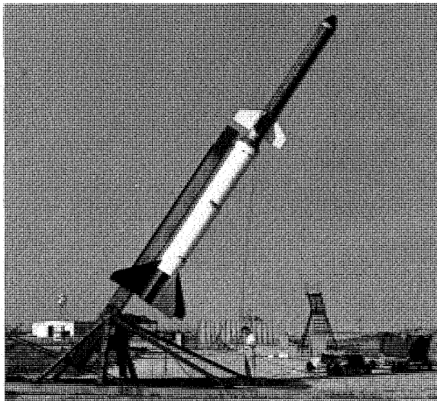
FIGURE 285. Project engineer Leo T. Chauvin examines firing leads to first Honest John-Nike launch vehicle used for heat-transfer test of blunt 50-degree cone. Vehicle is shown on Army Hermes launcher, ready for test at Wallops, September 15, 1955.
