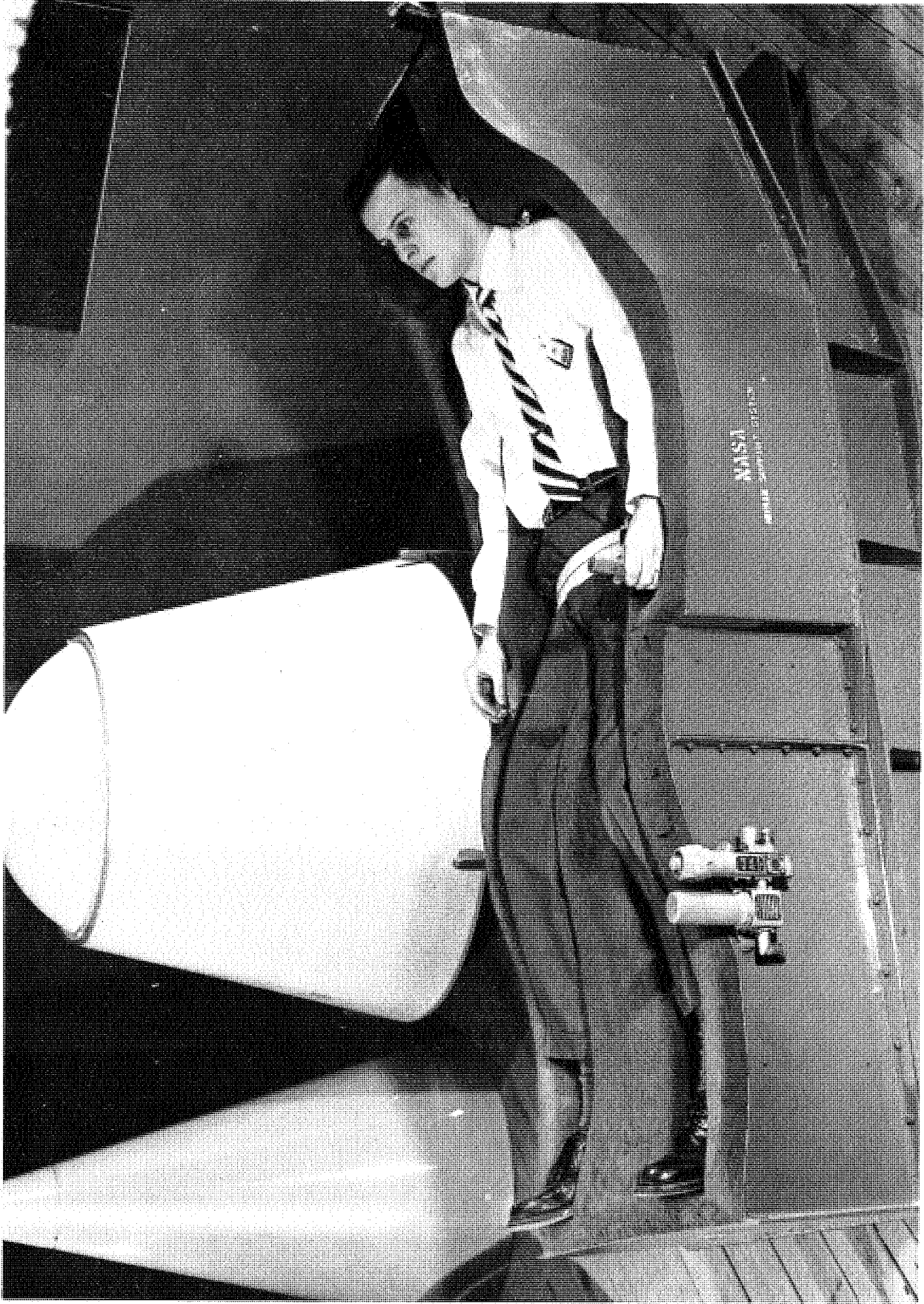
FIGURE 424. J. C. Heberlig demonstrates pilot position in first supine pilot-support system developed on Johnsville Centrifuge for Project Mercury.
