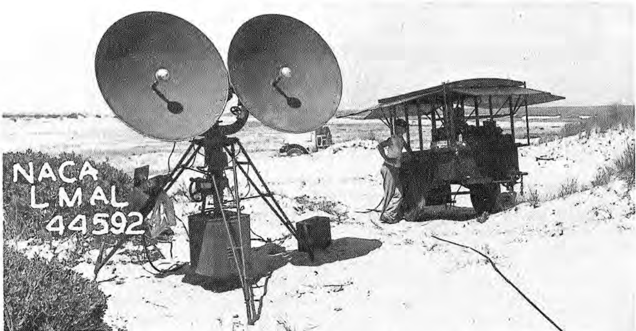
FIGURE 26. View of AN/TPS-5 radar at Wallops, June 1945. Engineer P. F. Fuhrmeister is shown beside the control van.
