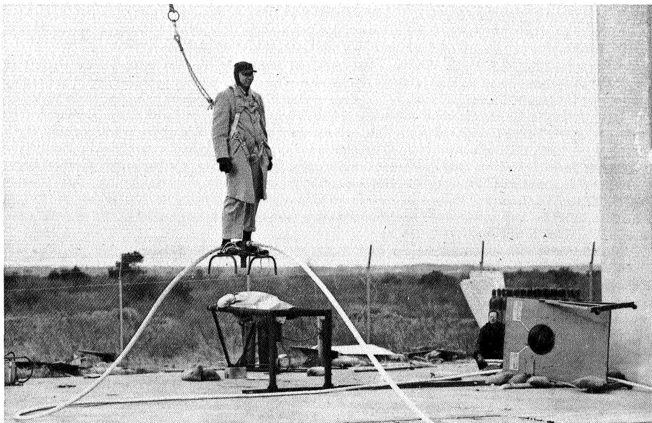
FIGURE 156. Paul R. Hill demonstrates ease of standing on Jet Board, and A. Spinak handles air-supply controls. Demonstration was given during visit of Air Force pilots, January 14, 1954.
