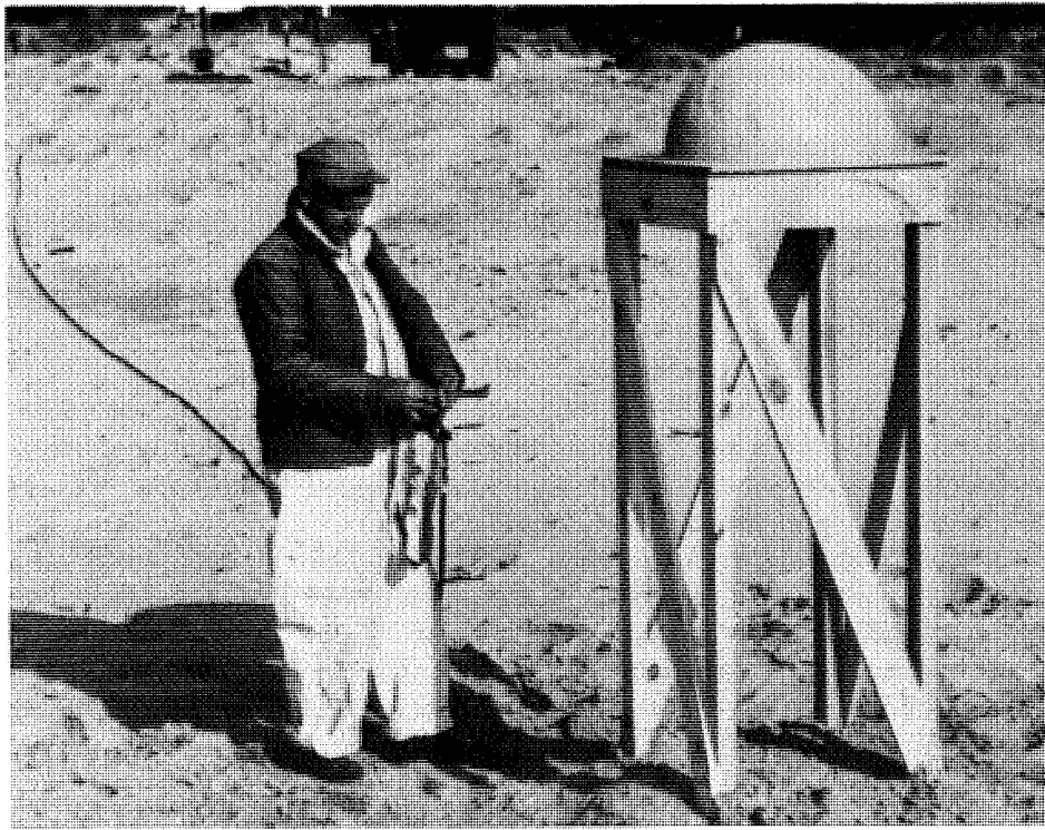
FIGURE 278. Technician E. R. Matthews connects firing leads to 150-pound hemispherical explosive charge in preparation for blast loads test, November 4, 1954.
