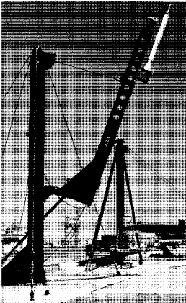
FIGURE 378. Test model of Polaris nose cone, shown on Recruit booster with flared base, April 14, 1958.
