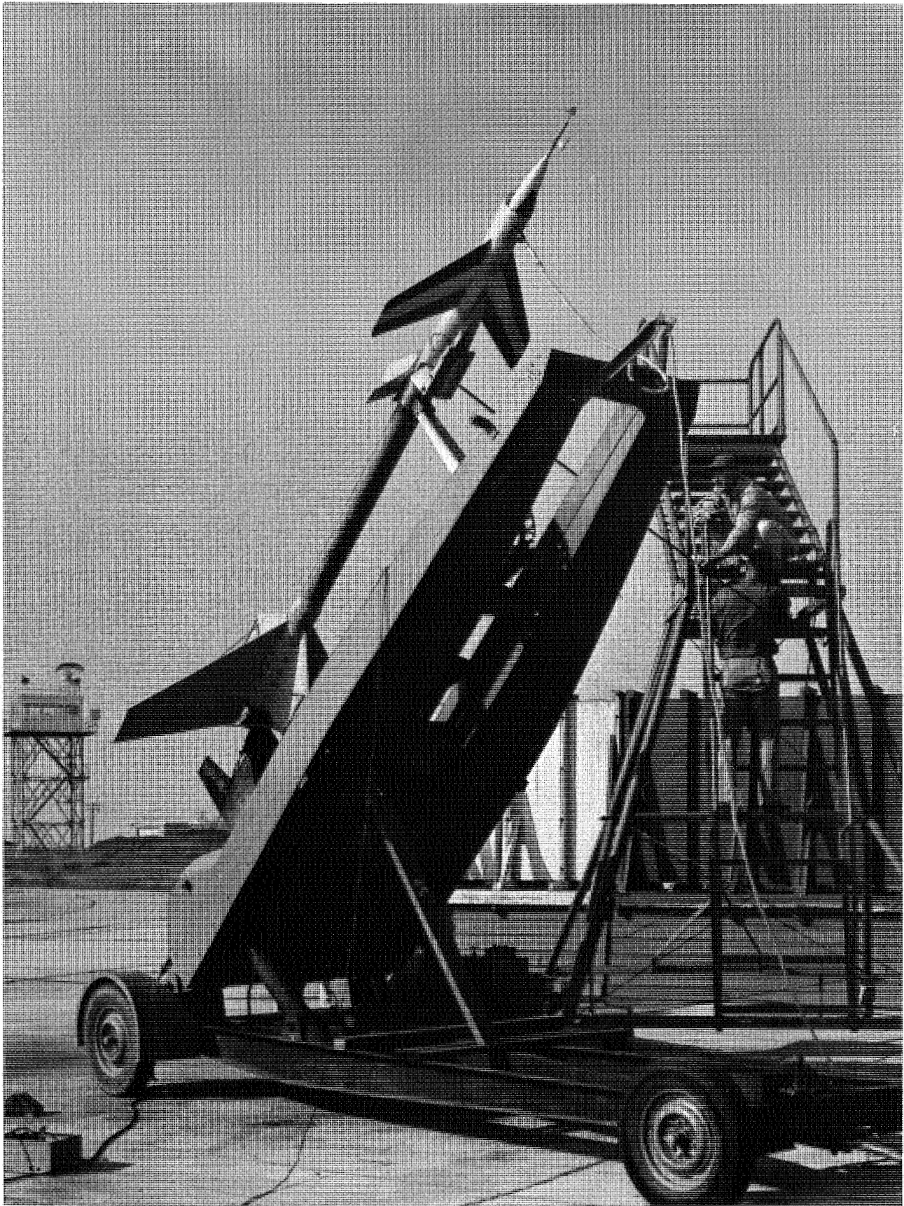
FIGURE 191. Technicians Durwood Dereng and Roy Hindle make final preparations for launch of model of McDonnell XF3H-1 airplane model with Deacon booster, June 10, 1953.
