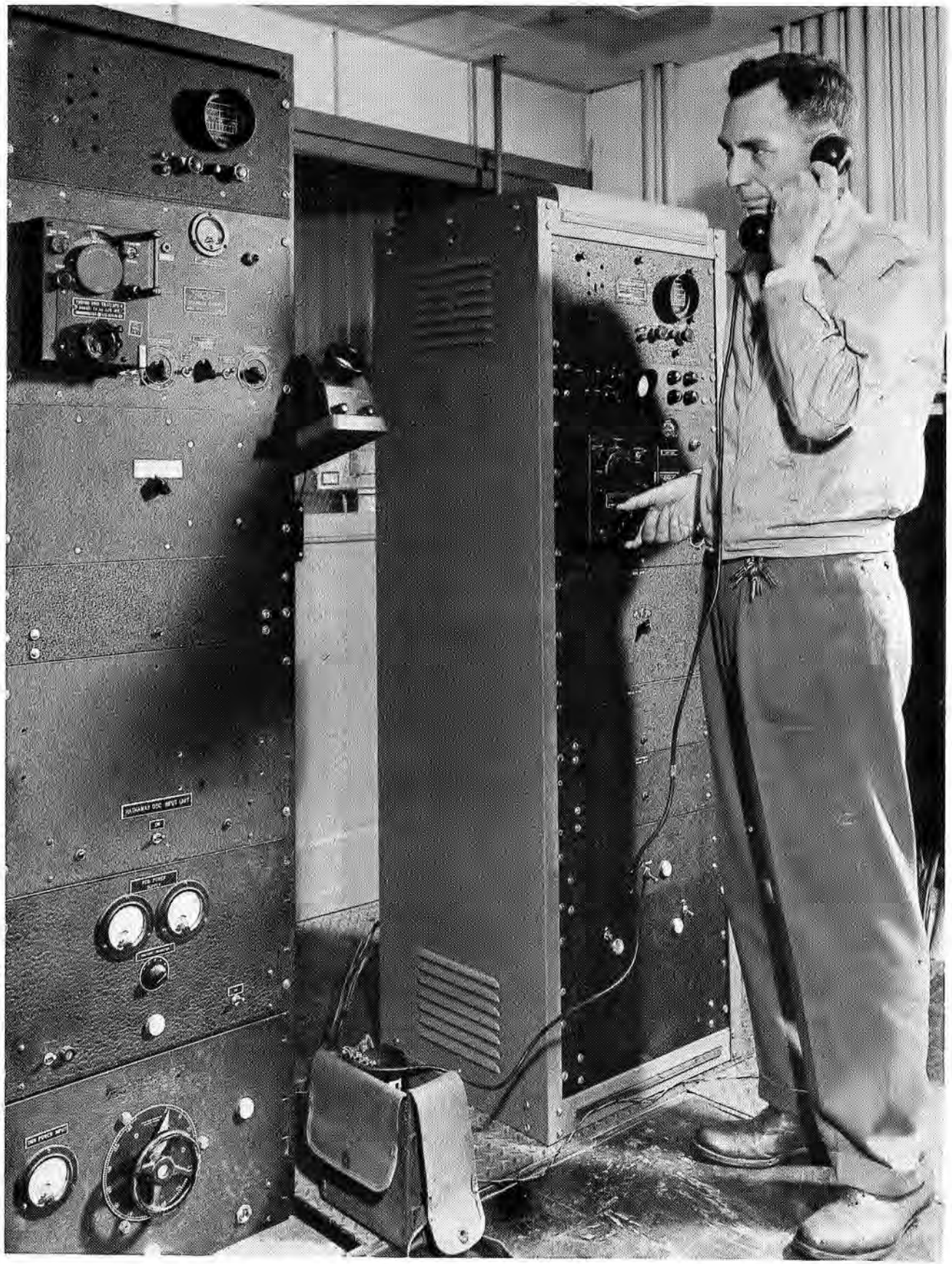
FIGURE 60. Engineer R. L. Hallett, Jr., listens over portable EE88 telephone as he adjusts spinsonde receiver during rocket test flight at Wallops Island, July 28, 1950.
