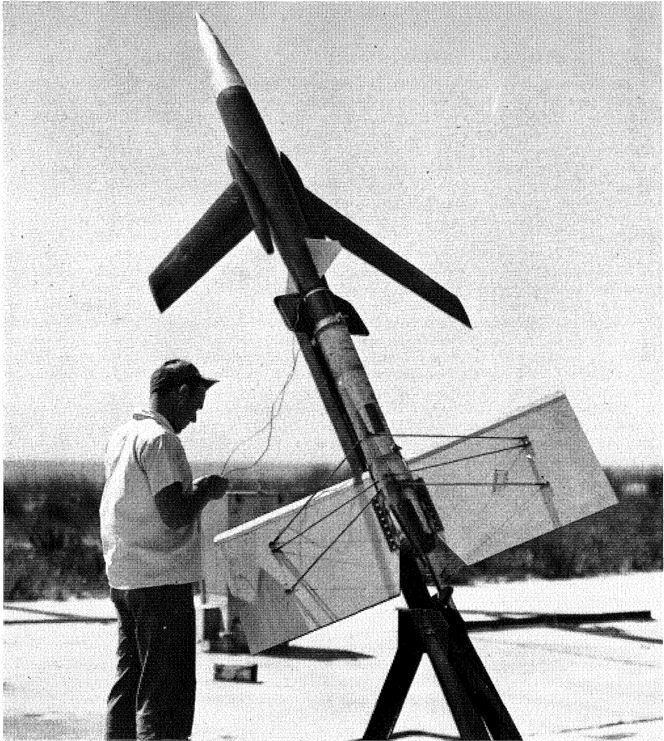
FIGURE 132. Technician Harry Bloxom connects firing leads on F25 model with inboard nacelles. Model is shown at Wallops on July 18, 1950.
